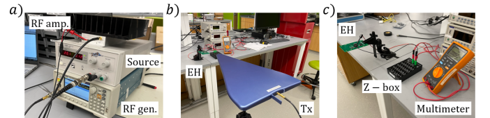
Fig. 4. Experimental setup, consisting in: a) RF generator and amplifier; b) transmitting directional, high-gain, broad-band antenna mounted on a tripod; and c) EH demo, located 0.5 m from the antenna. A manually tunable Z box is used as a load resistance ( R_{load} ) to calculate the rectified power. The voltage absorbed by Z_{load} is measured with a digital multimeter.
